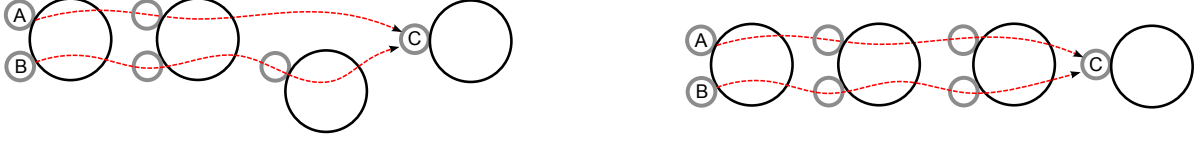
Fig. 2. Extracted feature examples from Traceroute measurements. (Left) - Out-degree match, where interface C has been observed on a down-path for both interface A and interface B ( i.e. , where observed paths exist where one path contains interfaces \{A, C\} and another path contains interfaces \{B, C\} ), and (Right) - Hop count match, where interface C has both been observed on a down-path for interface A and interface B and the hop count between the two (in this case, two hops) is the same for both.
